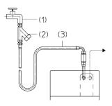
After the water stop cock (1), install a dirt trap (2) with a mesh width of 150 μm.
