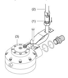
A water safety device (1) must be used in order for the softener to be operated in accordance with DIN requirements. A kit is available from Winterhalter for this purpose.
